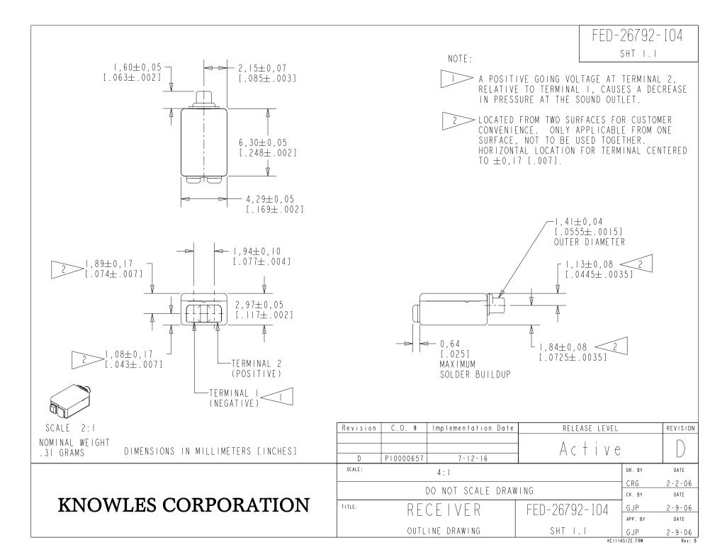
THE FED-26792-104 IS A FERROFLUID DAMPED ED-27305-000 WITHOUT TYPE III DAMPING WITH A PEAK OF 4dB RELATIVE TO THE SENSITIVITY AT IKHZ UNDER CONSTANT VOLTAGE DRIVE CONDITIONS. THIS MODEL HAS INCREASED DCR/IMPEDANCE RATIO.
